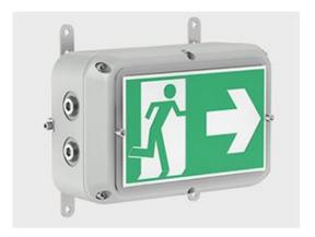
The SPARTAN Bulkhead Emergency Exit is designed specifically for hazardous environments which require high performance and high reliability. Using field-proven, long-life LED technology, SPARTAN Bulkhead Emergency Exit is IEC Ex certified for all Zone 1 and Zone 2 applications and rated for T4, T5 and T6 environments.
